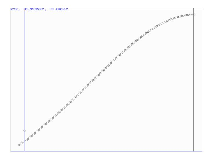
A very sharp "spike" occurs which will almost certainly be missed by a search algorithm, and indeed hardly shows on the graph! Sometimes these spikes can be predicted theoretically and a logical test for such cases is included in the algorithm.
