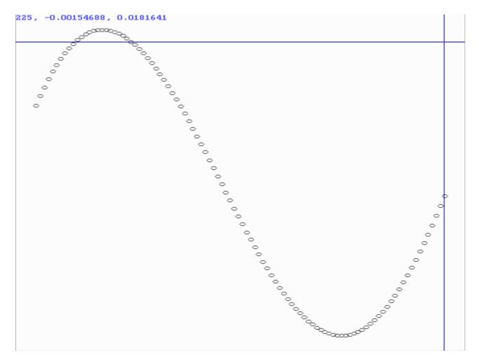
Here one or both of the two roots could be missed by the search. Incorporation of an analysis of changes in the gradient solved cases such as this. But the following graph shows a much more severe case:
